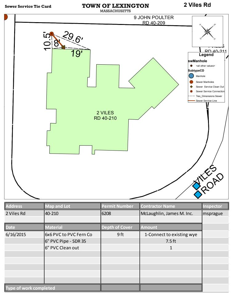
New 6" PVC sewer service installed to new house, connection to existing stub.
