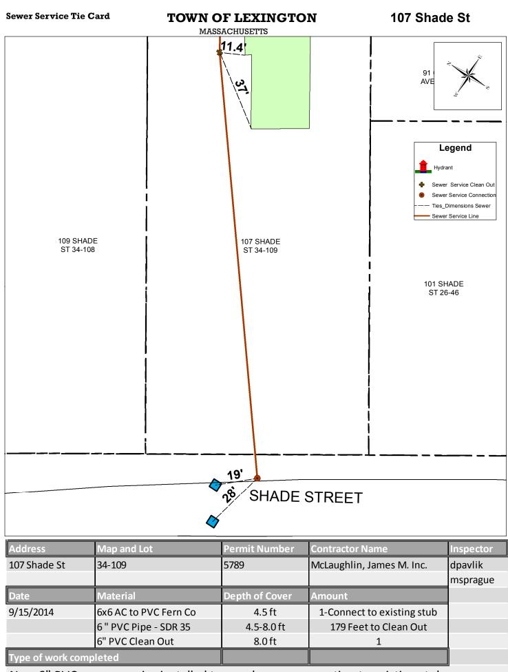
New 6" PVC sewer service installed to new house, connection to existing stub.
